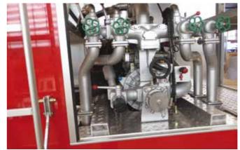
d) Electric driven: Low voltage (12 or 24 volt) DC electric motor driven rotary gear or eccentric vane primers are available in several compact versions. For the last 60 years, these were the most popular in North America. These primers are normally found in the middle price range.
